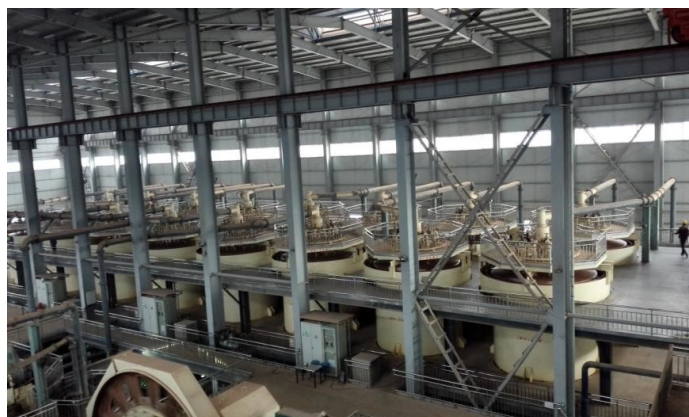
Figure 5. Application of non-drive flotation desilication technology for low-grade bauxite.
