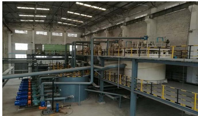
Figure 4. Application of flotation desulphurization technology for high-sulphur bauxite.
